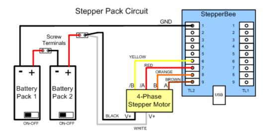
For ease of identification, the stepper motor has colour coded wires which correspond to those indicated in the circuit diagram above. The battery packs also use the traditional black for negative and red for positive terminals. It should be noted that each of the two battery packs supplied have their own on-off switch. Both packs must be switched on to operate the stepper motor. For those not familiar with circuit diagrams the following photo illustrates the connections.
